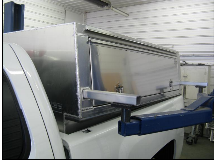
Lift-Off Receivers—4 Corners
